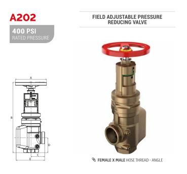
Used as a zone control valve for in-line application to regulate sprinkler, stand pipe and combined fire protection system. Indicator bonnet shows whether valve is opened or closed. Adjustuble scale permits easy field setting. The valve is used to regulate inlet pressure up to 400 lbs.
