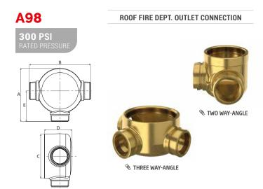
Used as a standpipe roof outlet connection by the fire service. Provides 250 GPM minimum per outlet. Used with straight or angle hose valves to provide water control.
