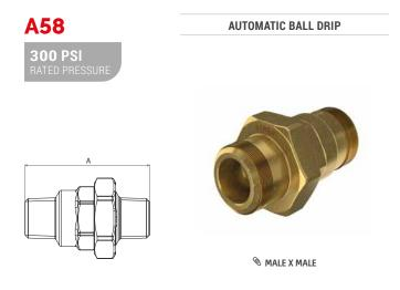
To drain low point of system between swing check valve and Fire Dept. connection. Automatically seals under pressure. Must be installed in horizontal position only.
