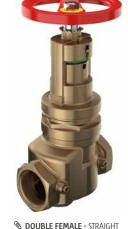
Used as a zone control valve for in-line application to regulate sprinkler, stand pipe and combined fire protection system. Indicator bonnet shows whether valve is opened or closed. Adjustuble scale permits easy field setting. The valve is used to regulate inlet pressure up to 400 lbs.
