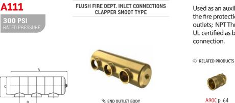
Used as an auxiliary inlet connection to supplement the fire protection water supply. Available with 3, 4, 6 outlets; NPT Threads. Made of forged brass. UL certified as both roof manifold and flush fire dept. connection.
