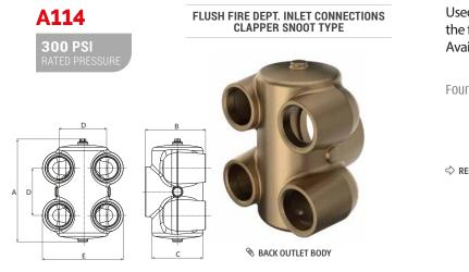
Used as an auxiliary inlet connection to supplement the fire protection water supply. Available with NPT Threads. Casted bronze.
