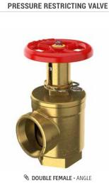
Used with a fire hose rack assembly. Water pressure is controlled by adjustable flow restriction. If full flow is required, the restriction may be overridden.
